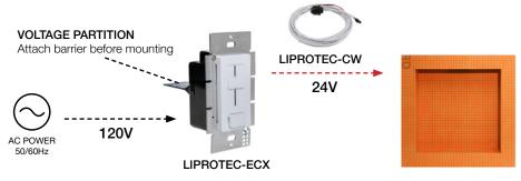
Note: Main power (120V source power) must come through the bottom of the switch box.
