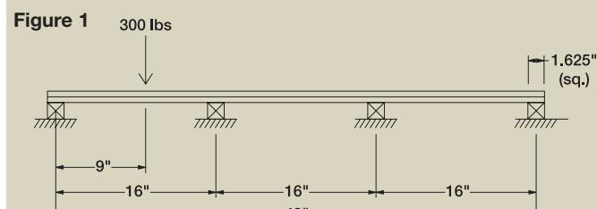
Cross-sectional view of the test specimen assembly for the Robinson-Type Floor Tester with applied load creating maximum moment on the floor sheathing layers.
