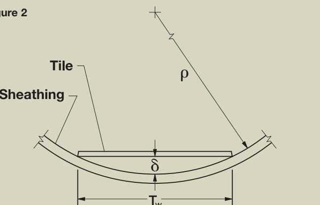
The tile and sheathing interface model showing an exaggerated gap between the single tile and the floor sheathing.
