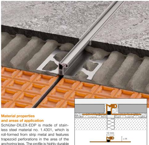
Schlüter-DILEX-EDP is made of stainless steel material no. 1.4301, which is roll-formed from strip metal and features trapezoid perforations in the area of the anchoring legs. The profile is highly durable and especially suited for application areas that must be resistant to chemicals and acids, such as the food industry, breweries, dairies, industrial kitchens, and hospitals as well as residential spaces.
