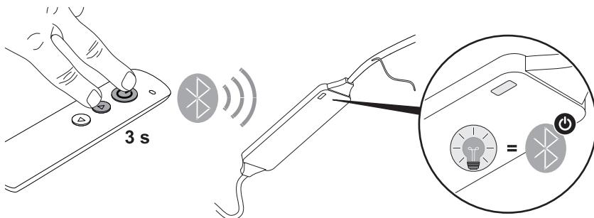
To make it possible for the Bluetooth receiver to establish a Bluetooth connection with a mobile device (Bluetooth pairing), the pairing readiness needs to be activated via the radio remote control. If the Bluetooth receiver is to be controlled using a mobile device, the Schlüter®-LED-COLOR-CONTROL app needs to be installed » "Schlüter®-LED-COLOR-CONTROL" on page 60.
