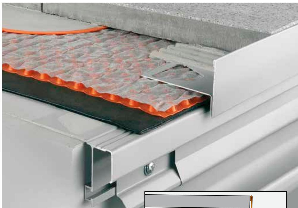
upper edge of the profile. TROBA-PLUS must be installed as an area drainage membrane between the waterproofing layer and the screed to ensure that water cannot accumulate in the screed layer.
