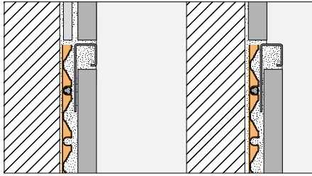
Installation variant: Wall edging profile Schlüter®-QUADEC
