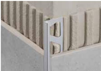
Schlüter-JOLLY are decorative metal profiles to finish and protect tiled external wall corners and other tiled edges, e.g. tiled skirting. The 90 degree angled finishing leg safeguards tiles against mechanical damage. The joint spacers on both sides create a uniform grout joint with the tile. The geometric profile undercutting offers additional bonding surface for the grout. The innovative plug-in connection of the corner pieces results in neat, visually appealing corner formations.
