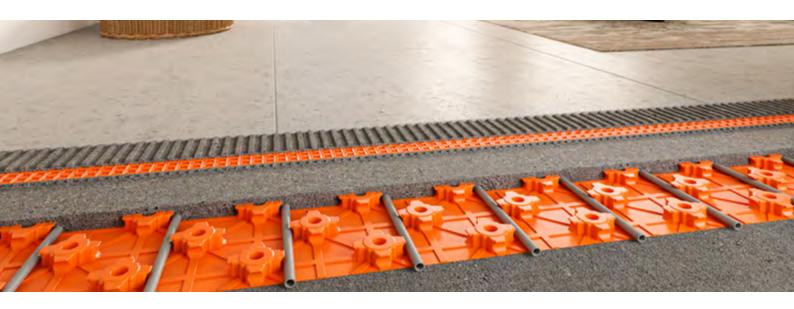
Schlüter®-BEKOTEC-THERM is an innovative solution for creating heated tiled floors. Our proven system, including innovative studded screed panels, is quickly installed without using costly, construction materials – ceramic tile coverings can typically be installed just one day after a 4:1 sand:cement screed (with NO fibres or reinforcements) has been installed on top of the studded screed panels.
