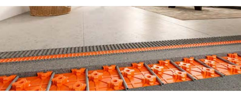
Schlüter®-BEKOTEC-THERM is an innovative solution for creating heated tiled floors. Our proven system, including innovative studded screed panels, is quickly installed without using costly, construction materials – ceramic tile coverings can typically be installed just one day after a 4:1 sand:cement screed (with NO fibres or reinforcements) has been installed on top of the studded screed panels.
