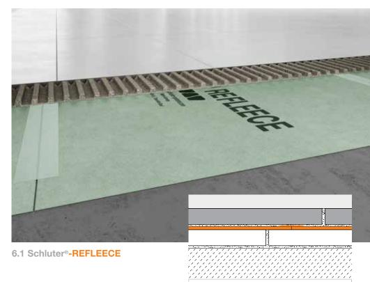
Tiles installed on the REFLEECE should be at least 4" x 4" (10 cm x 10 cm) and have a minimum thickness of 1/4" (6 mm).
