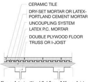
Floors, Interior Wood Subfloor, 24" o.c. Joist Spacing, with Uncoupling System Latex-Portland Cement
