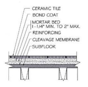
Floor, Interior Wood Subfloor Cement Mortar
