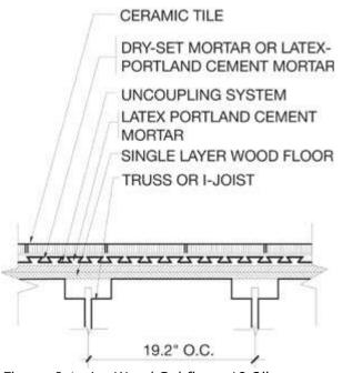
*Floors, Interior Wood Subfloor, 19.2" o.c. Joist Spacing, with Uncoupling System Latex-Portland Cement*
