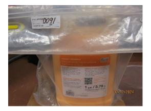
California 01350/ASTM D5116 Small Chamber Tests for Volatile Organic Compound Emissions From Products
