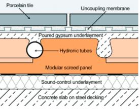
The modular screen assembly helps ensure durability of the tile covering, optimizes radiant heat transfer to the space and reduces sound impact transmission.
