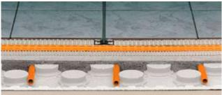
The studs on the modular screed panel limit curing stresses and form a grid pattern to hold the hydronic heating tubes.
