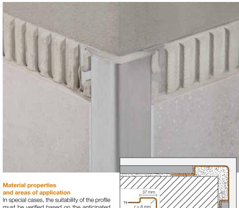
In special cases, the suitability of the profile must be verified based on the anticipated chemical and mechanical stresses.
