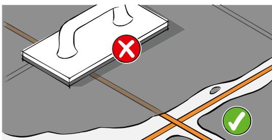
No grouting around profile and insert
