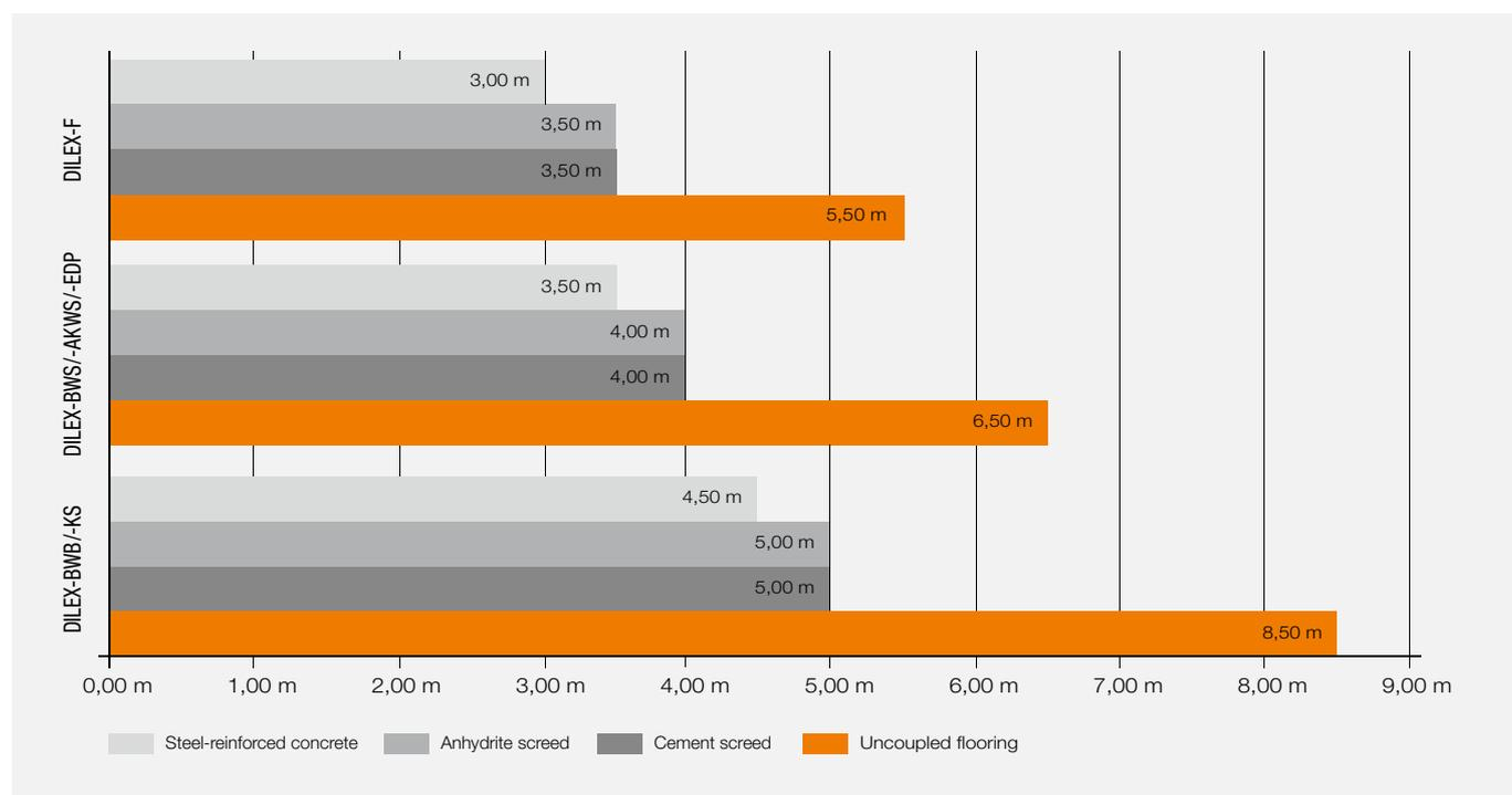
\* tiled segment sizes were determined with the above formula, using a mean expansion coefficient for each structural component and a safety factor of 0.6. The result was then rounded to 0.5 m.
