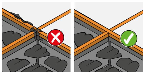
Any excess tile adhesive must be removed immediately.
