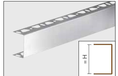
Schlüter-KERDI-BOARD-ZB is a U-shaped profile of stainless steel with three sided perforation. It is used for fastening and stabilising structures made of Schlüter-KERDI-BOARD panels.
